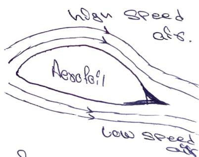
An Aeroplane uses aerofoil for lifting. Upper surface of aerofoil is made more curved than the lower surface because of which air flows faster over the upper surface compared to lower surface which creates low pressure at the upper surface and high pressure at the lower surface, which lifts up the aeroplane.
